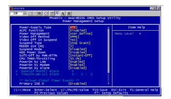
Figure 3.7: Power management setup screen (1)
